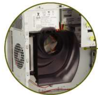
CAG1.1 Air Duct
